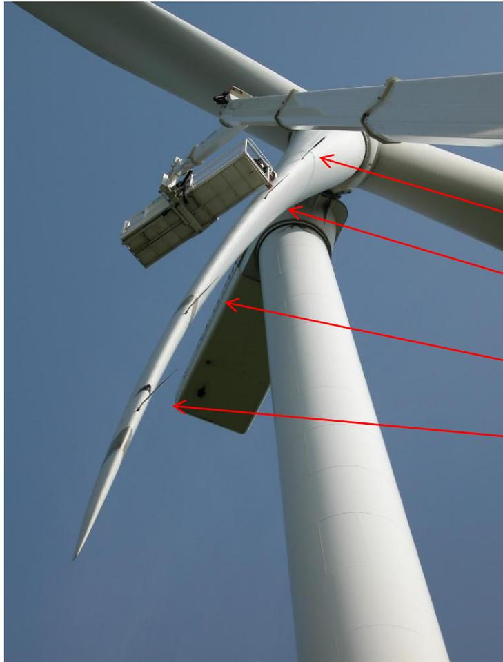
Normal force measured at four radial positions by pressure holes
