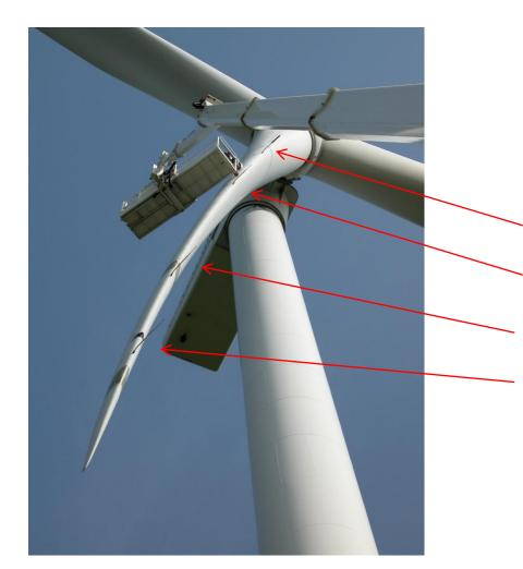
Normal force measured at four radial positions by pressure holes
