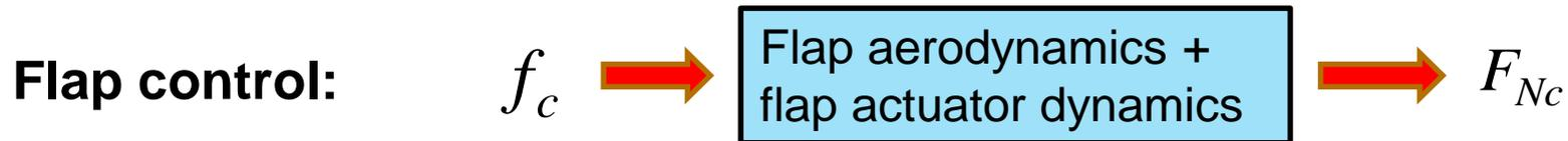
The flap control is numerically simulated by the aeroelastic code HAWC2 where the flap aerodynamics and flap actuator dynamics are modeled
