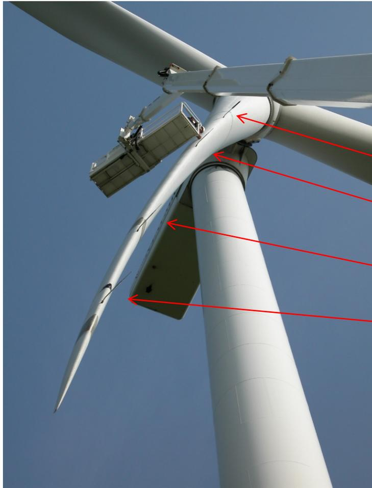
Four 5 hole pitot tubes installed on a NM80 turbine with an 80m rotor
