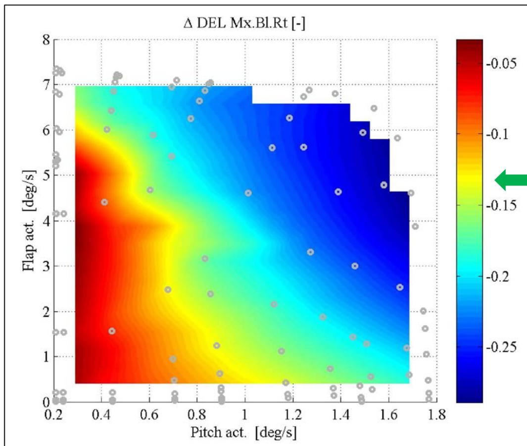
Fatigue Damage Equivalent Loads (DEL) alleviation at the blade root flapwise bending compared to the baseline NREL 5 MW turbine, Wöhler curve exponent of 10.
