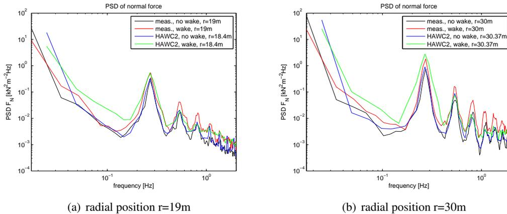
Figure 7: PSD of the blade normal force.
