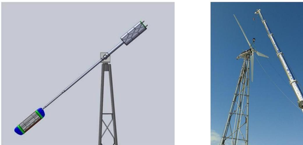
Figure 9 To the left is shown the principal layout of the rotating test rig. To the right is shown the 100 kW Tellus turbine at DTU, Campus Risoe which will be used as the basic platform for the rotating test rig.
