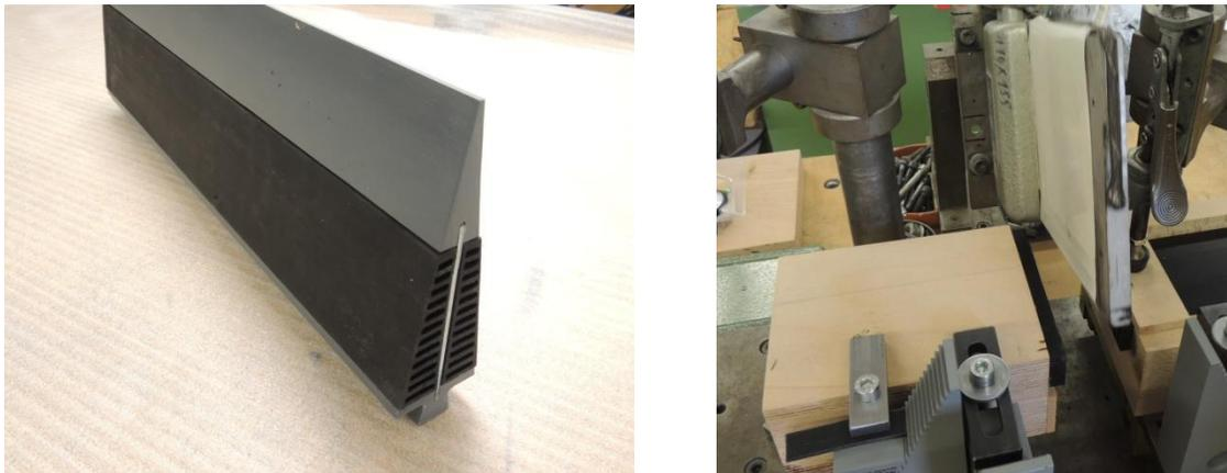
Figure 4 To the left is shown the components of the flap before gluing the parts together. To the right the contact welding of the end caps is carried out.
