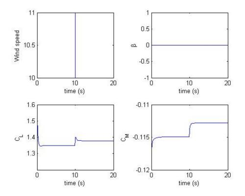
Figure 2 The wind step is shown in the upper left graph. There is no active control as seen in the upper right graph. The lower left graph shows  $C_L$  response and the lower right graph shows the  $C_M$  response.
