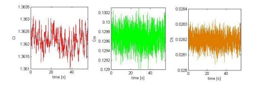
*Figure 16 Response of system for a turbulent wind speed input – Feedback control of TE flap (zoom in).*
