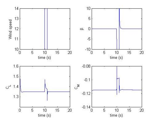
Figure 5 The wind gust is shown in the upper left graph. The active control is seen in the upper right graph. The lower left graph shows  $C_L$  response and the lower right graph shows the  $C_M$  response.
