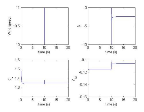
Figure 3 The wind step is shown in the upper left graph. The control is active and the flap deflection is seen in the upper right graph. The lower left graph shows  $C_L$  response and the lower right graph shows the  $C_M$  response.
