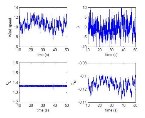
Figure 7 A turbulent wind series is shown in the upper left graph. The active control is seen in the upper right graph. The lower left graph shows  $C_L$  response and the lower right graph shows the  $C_M$  response.
