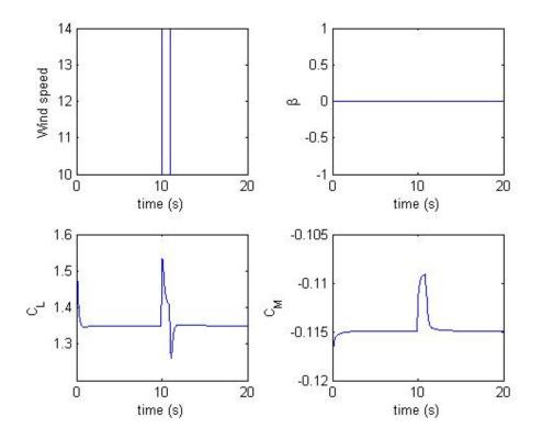
Figure 4 The wind gust is shown in the upper left graph. There is no active control as seen in the upper right graph. The lower left graph shows  $C_L$  response and the lower right graph shows the  $C_M$  response.
