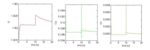
Figure 10 Response of system for a step in wind speed – Feedback control of TE flap (zoom in)
