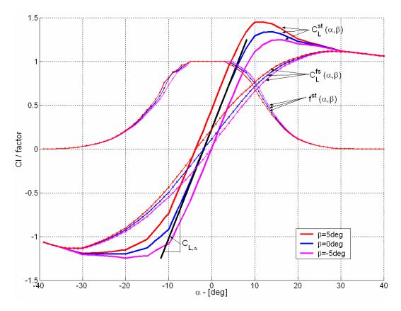
Figure 1 Example of a static lift curves for ATEG deflection for  $\beta = -5$ , 0 and 5 degree.
