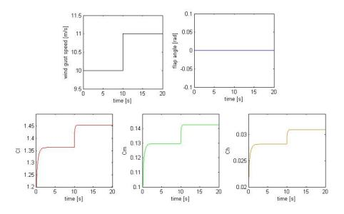
Figure 8 Inputs and response of system for a step in wind speed – No control of TE flap
