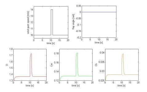
*Figure 11 Inputs and response of system for a square wind speed input – No control of TE flap*
