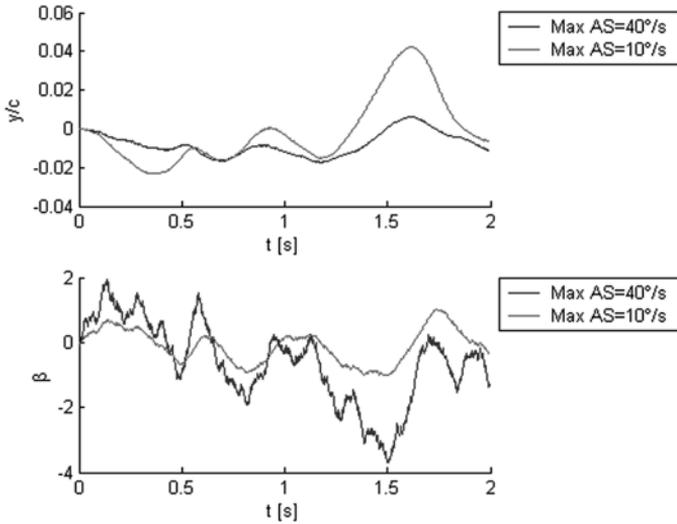
Figure 8: Displacements and flap deflections as function of time for two different maximum actuation speeds
