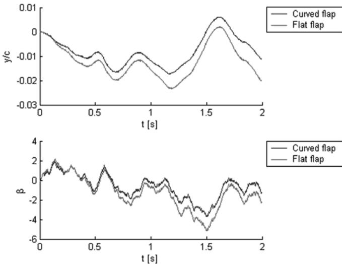
Figure 7: Displacements and flap deflections as function of time for curved and flat flap
