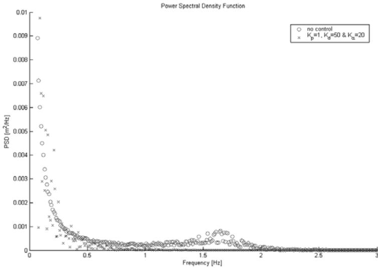
Figure 6: Power spectra density of the displacements as function of frequency for *no control* vs. *controlled*
