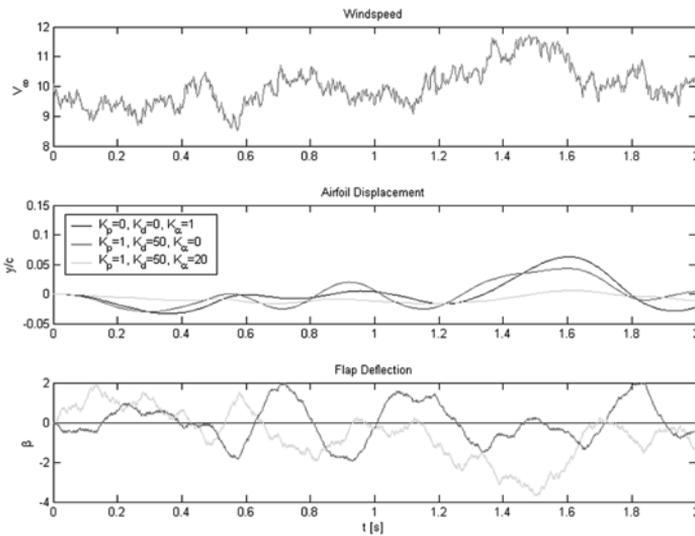
Figure 5: Displacements and flap deflections as function of time, 100 s simulations
