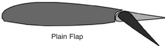
Figure 2: Schematic of airfoil with trailing edge flap
