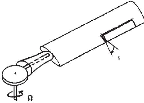
Figure 1: Schematic of blade with trailing edge flap
