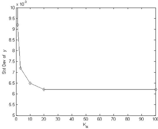
Figure 3: Sensitivity of the system response to  $K_\alpha$  measured as standard deviation of oscillation and AS not limited
