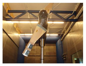
Fig. 2. Photo of the "smart" blade equipped with actuators and sensors.
