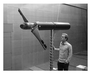
Fig. 1. Photo of the "smart" two-bladed turbine with the trailing-edge flaps. The person standing next to it illustrates the size of the system.
