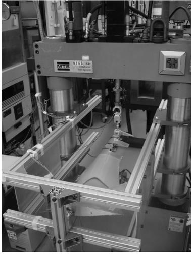
Figure 2: Blade testing set-up
