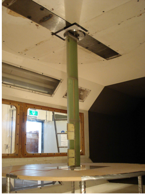
Figure 1. The adaptive blade at the TU Delft LSLT wind tunnel test section.
