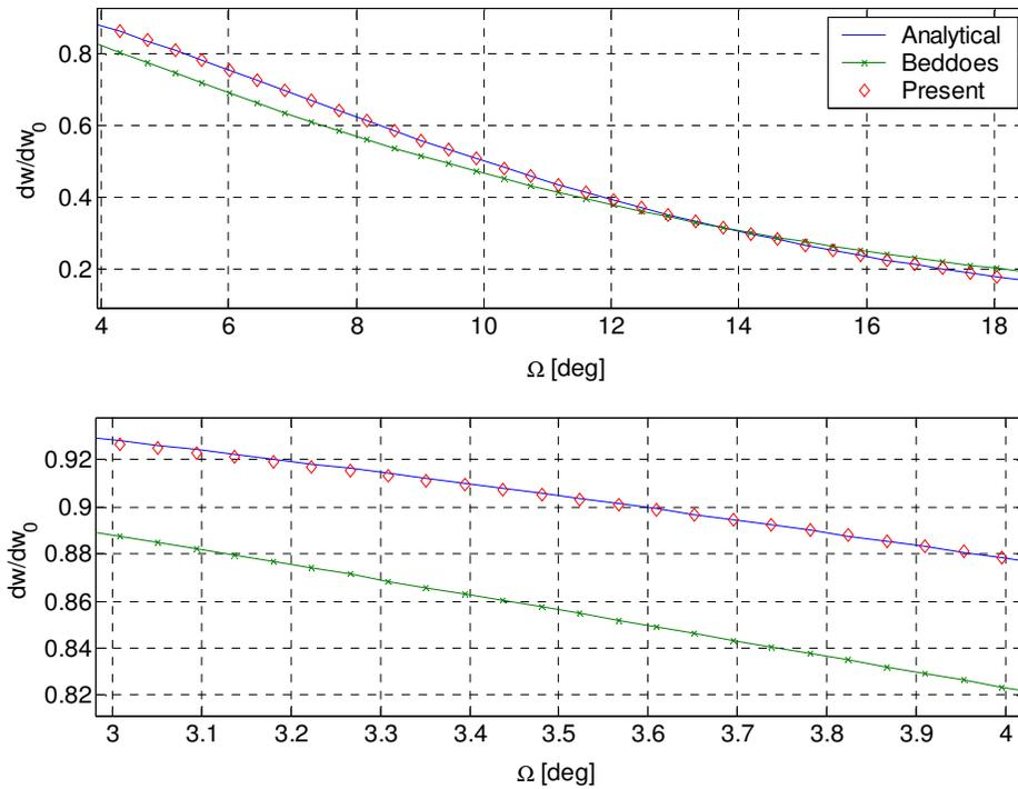
Figure 3; illustrates a comparison of the downwash decay rate for  $h/r=-0.275$  between the analytical solution from Equation (2), Beddoes two term exponential approximation and the presented exponential approximation for  $n=6$ .
