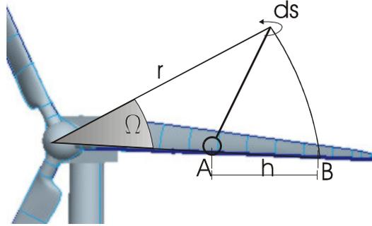
Figure 1; model geometry for the near wake model, azimuth angle is  $\Omega$ , distance between two points A,B on blade is  $h$  and the length  $ds$  of a trailed vortex element at radius  $r$  contributing to the induction at point A.
