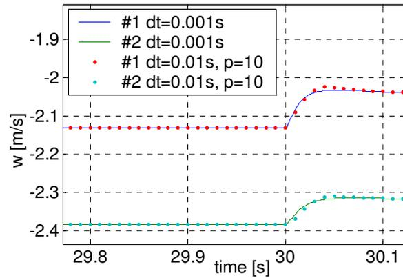
Figure 5; illustrates step changes in axial induction for two radial positions calculated with time steps of 0.001 second and 0.01 second length but with the domain subdivided in 10 equal portions ( $p=10$ )
